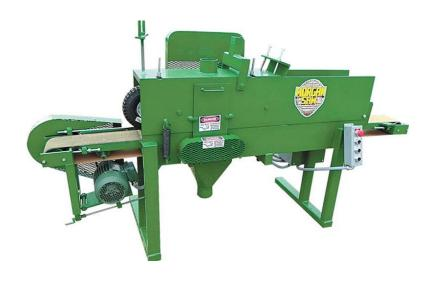
The Morgan Board Deduster manufactured by Sawmill Supplies and Equipment is designed to quickly dedust board free of loose material. Equipped with two brushes to remove dust in one pass. Constructed of heavy gauge structural tubing and heavy 1/4" plate.
